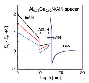
FIG. 3. (Color online)  $E_{\rm C}$  potential profiles of the In<sub>0.17</sub>Al<sub>0.83</sub>N (10 nm)/Al<sub>0.38</sub>Ga<sub>0.62</sub>N (5 nm)/AlN (0.75 nm)/GaN structure calculated for several  $E_{\rm F~surf}$  positions.
