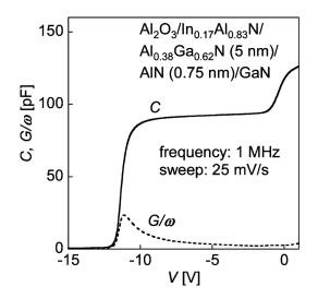
FIG. 2. Measured C-V curve for the Al<sub>2</sub>O<sub>3</sub> (10 nm)/In<sub>0.17</sub>Al<sub>0.83</sub>N (10 nm)/Al<sub>0.38</sub>Ga<sub>0.62</sub>N (5 nm)/AlN (0.75 nm)/GaN structure.  $C_i$  was estimated to be ~260 pF. The bias voltage was swept from the positive side to the negative side at a sweep rate of 25 mV/s.
