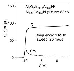
FIG. 6. Measured C-V curve for the Al<sub>2</sub>O<sub>3</sub> (13 nm)/In<sub>0.18</sub>Al<sub>0.82</sub>N (12 nm)/Al<sub>0.44</sub>Ga<sub>0.56</sub>N (1.5 nm)/GaN structure.  $C_i$  was estimated to be ~190 pF. The bias voltage was swept from the positive side to the negative side at a sweep rate of 25 mV/s.
