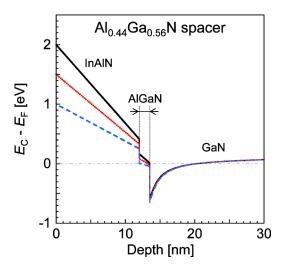
FIG. 5. (Color online)  $E_{\rm C}$  potential profiles of the In<sub>0.18</sub>Al<sub>0.82</sub>N (12 nm)/Al<sub>0.44</sub>Ga<sub>0.56</sub>N (1.5 nm)/GaN structure calculated for several  $E_{\rm F}$  surf positions.
