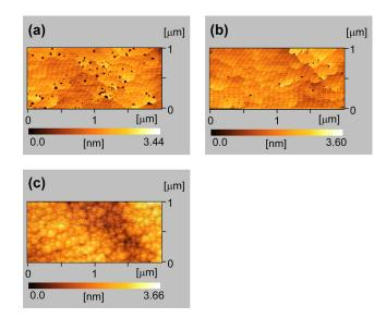
FIG. 4. (Color online) AFM images for (a)  $Al_{0.44}Ga_{0.56}N$  (2.0 nm)/GaN, (b)  $Al_{0.44}Ga_{0.56}N$  (1.5 nm)/GaN, and (c)  $In_{0.18}Al_{0.82}N$  (12 nm)/ $Al_{0.44}Ga_{0.56}N$  (1.5 nm)/GaN.
